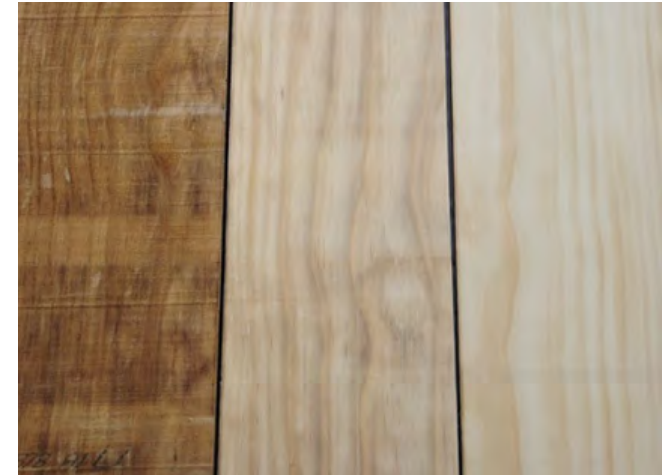
DISCOLORATION: ROUGH BOARD, AFTER SURFACING 1/8 INCH AND AFTER SURFACING 1/4 INCH FROM ROUGH
